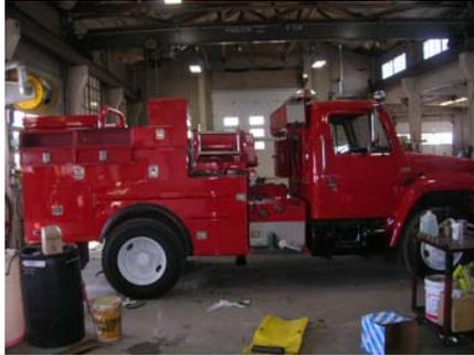
The Type III unit seats six, has a 500-gallon water tank, and has a hydrostatically-driven pump (allowing the vehicle to pump while moving). Compartments are designed to carry a variety of hand tools specific for wildland use. The low center of gravity helps to ensure safe operations in a variety of terrain types.
