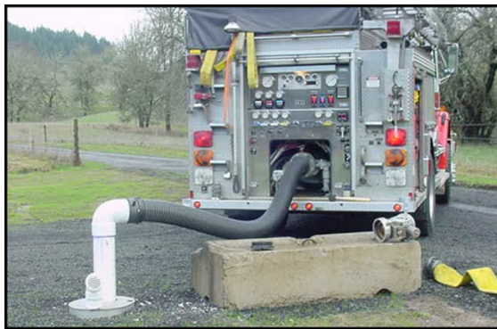
Tender using a hydrant to fill its tank
